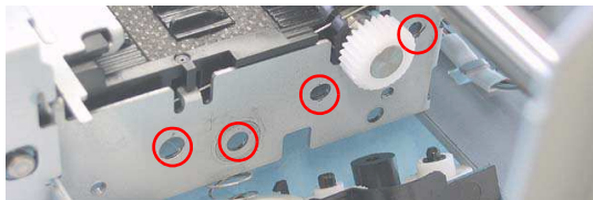
Figure 4-71. Reinstalling the Ink System (1)
