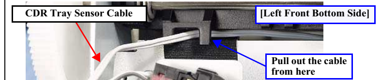
Figure 4-111. Routing the CDR Tray Sensor Cable
