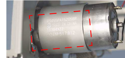
Figure 4-87. Reinstalling the CR Motor
