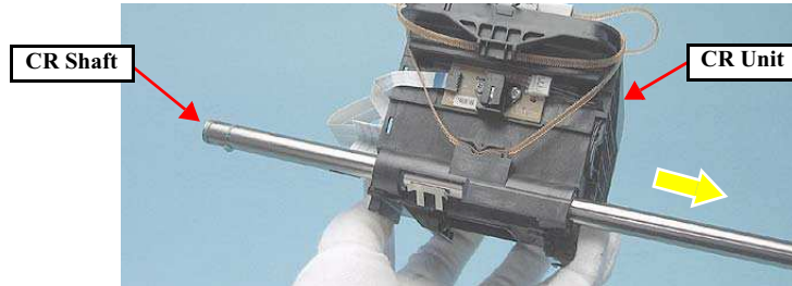
Figure 4-91. Removing the CR Unit (4)
